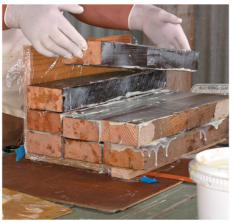
**STEP 4** You have about 45 minutes to glue the blocks together. Butter the glue to an edge and top surface of the first piece and put in place. Apply glue to 2 edges and a flat of the next piece and add it to the first. Always place glue to glue. Don't rely on glue from 1 piece binding it to an adjacent piece. After you have put down 2 layers, add glue to the tops before you add the next layer.
