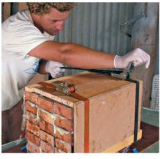
**STEP 5** Once all pieces are properly positioned, wrap the block in cling wrap, then sit the other corner form on the opposite corner. Bring straps over the top, and, if necessary, place an extra spacer, pieces of scrap timber (40 x 19m), where
