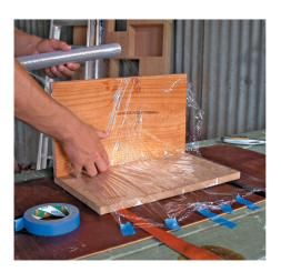
**STEP 2** Lay the thin plywood on your bench for protection, then lay out the ratchet straps about 350mm apart. On top of these, place the corner form, then cover its surface and a little beyond with cling wrap. Tape the cling wrap to the bench to make it easier to handle.
